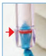
Complete filling by pulling down on the plunger until **red O-ring** is below the ridge (fill line).
